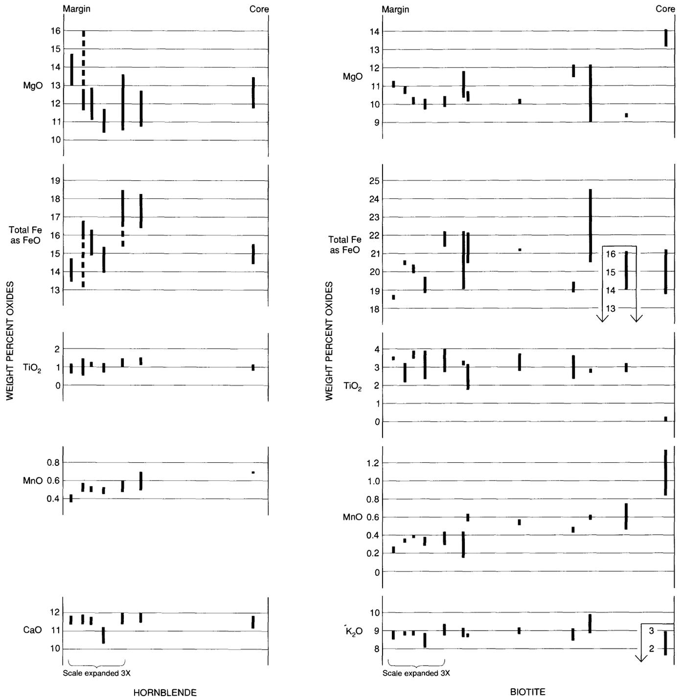
FIGURE 10.—Composition of hornblende and biotite in samples collected from margin to core of compositionally zoned bulbous head at north end of the Mount Givens Granodiorite. Dashes indicate range in one or two determinations for several samples. From Bateman and Nokleberg (1978).
