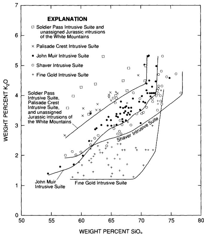
FIGURE 49.—Variation of  $K_2O$  with  $SiO_2$  in representative intrusive suites. For each intrusive suite, solid curves are drawn at lower limit of weight percent  $K_2O$  (excluding aberrant data points).  $K_2O$  increases successively eastward in suites, whereas  $SiO_2$  ranges from about 50 to 75 weight percent in all suites.
