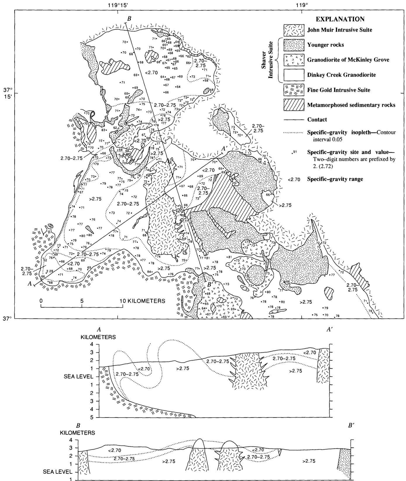
FIGURE 37.—Generalized geology and variations in specific gravity of the Dinkey Creek Granodiorite and associated rocks. Cross sections are conjectural.
