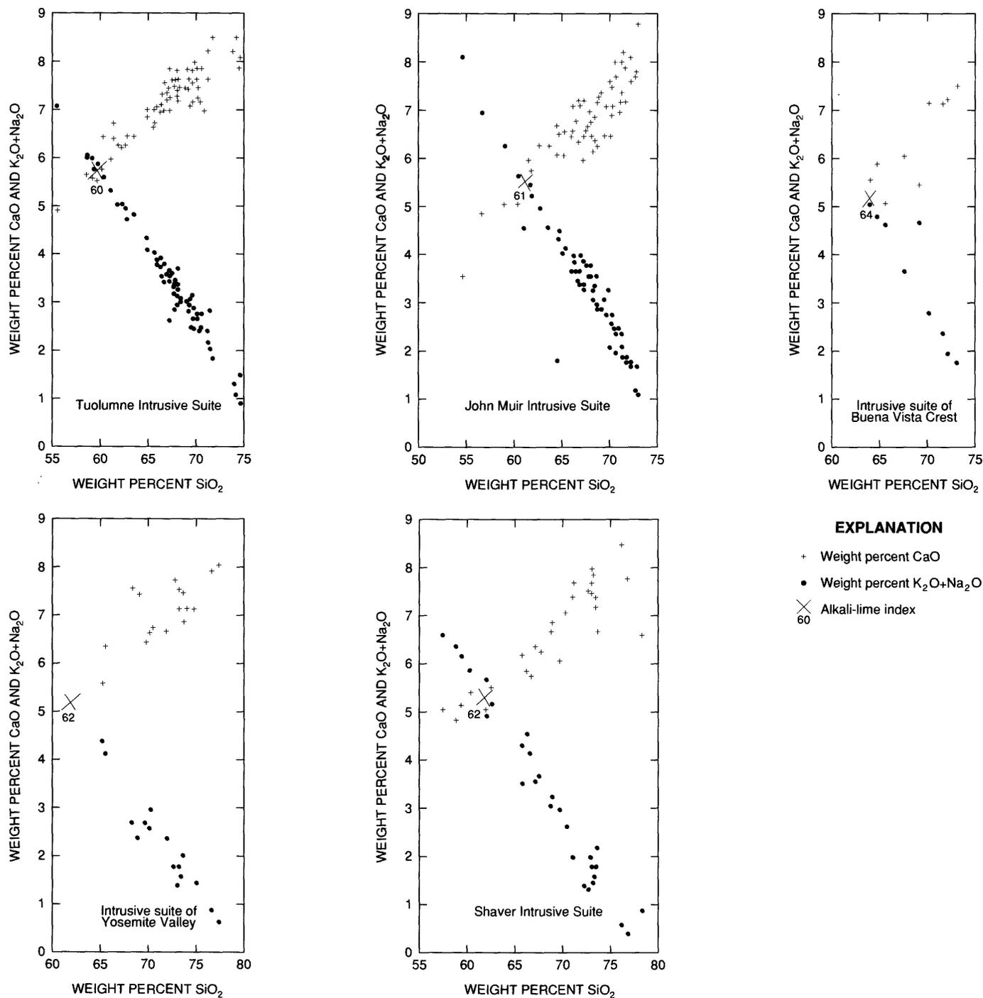
FIGURE 50.—Alkali-lime (Peacock) index values for intrusive suites. Index is weight percent  $\text{SiO}_2$  where weight percent  $\text{CaO}$  equals weight percent  $\text{K}_2\text{O}+\text{Na}_2\text{O}$  (Peacock, 1931). Figure continued on following page.
