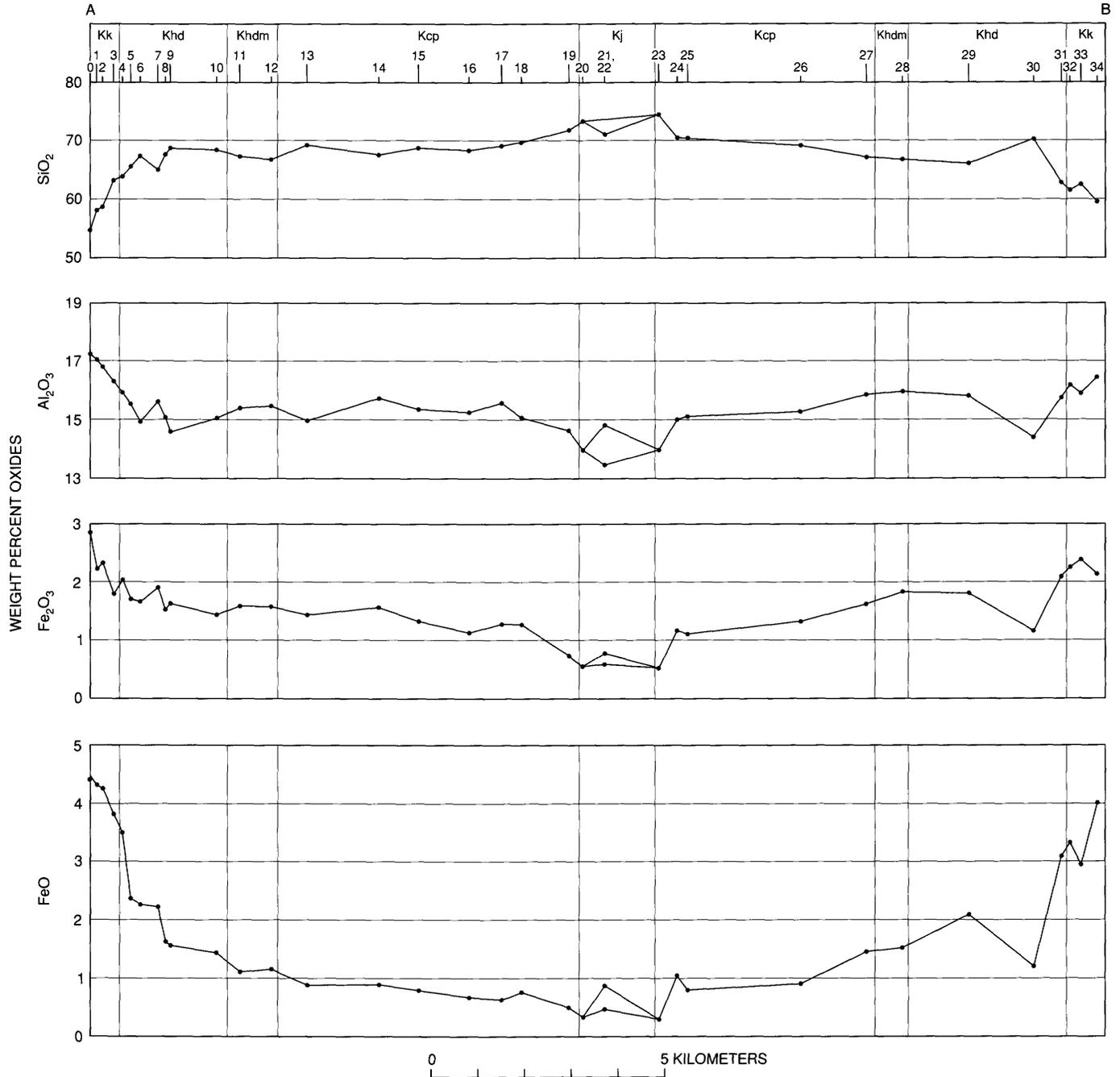
FIGURE 35.—Variations in major oxides along traverse A-B (fig. 32) across the Tuolumne Intrusive Suite. Kk, granodiorite of Kuna Crest and other granitoids in margins of batholith; Khd, equigranular facies of the Half Dome Granodiorite; Khdm,
