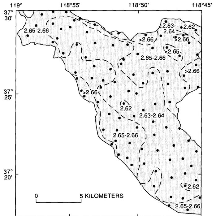
FIGURE 80.—Variations in specific gravity within central and southern parts of the Mono Creek Granite. Dots show sample localities; dashed lines separate areas of different specific gravity. Modified from Lockwood (1975).
