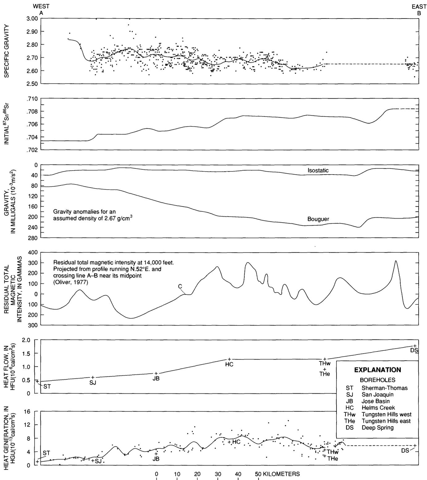
FIGURE 57.—Specific-gravity, initial  $^{87}\text{Sr}/^{86}\text{Sr}$ , and geophysical data across Sierra Nevada along line A-B (fig. 45). Initial  $^{87}\text{Sr}/^{86}\text{Sr}$  data from Kistler and Peterman (1973). Residual total magnetic-intensity curve (at 4,267 m) is projected from profile that strikes N.  $52^\circ$  E. (Oliver, 1977) and crosses line
