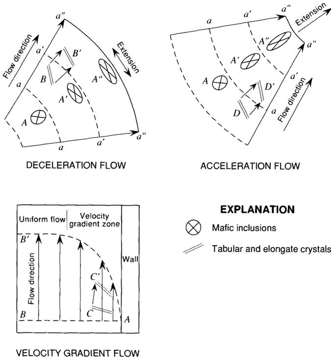
FIGURE 12.—Three types of nonuniform flow that can produce foliation and lineation in plutonic rocks. Diagrams represent either horizontal or vertical sections. Modified from Mackin (1947). See text for discussion.
