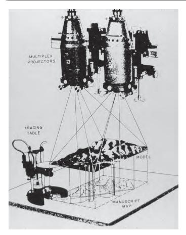
**Figure 25.** Convergent photography for map production employed stereoscopic models projected onto a tracing table. This allowed elevations to be determined with more accuracy, and at less cost, than former methods.
