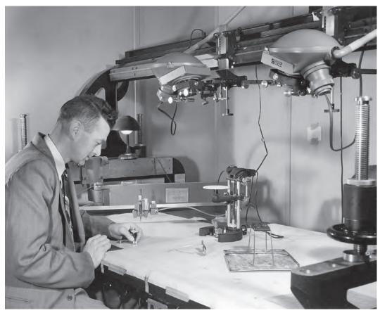
**Figure 26.** Russell K. Bean of the U.S. Geological Survey patented the ER–55 stereoplotting instrument, which proved superior to the Multiplex plotter in the compilation phase of topographic mapping.
