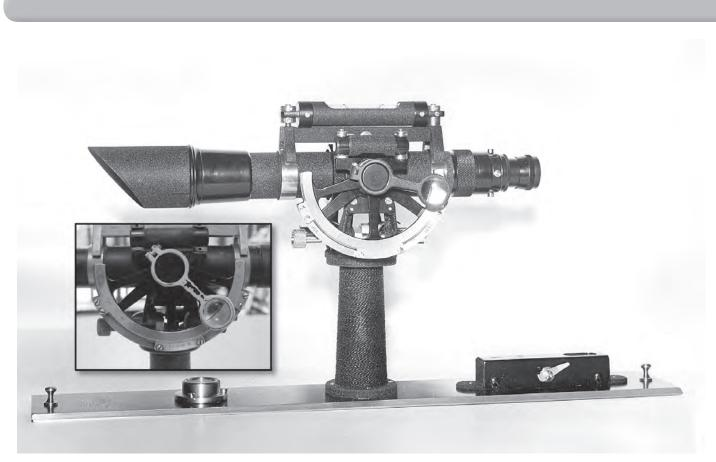
**Figure 18.** A Keiffel & Esser high standard alidade was used in conjunction with a plane table. The inset shows detail of W.M. Beaman's (U.S. Geological Survey topographer) improvement to the instrument, the Beaman Arc.
