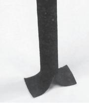
**Figure 15.** When a structure was not available for cementing a stemmed disk, a 4-foot long wrought iron post with a bronze bench mark cap riveted to the top was planted by survey crews.
